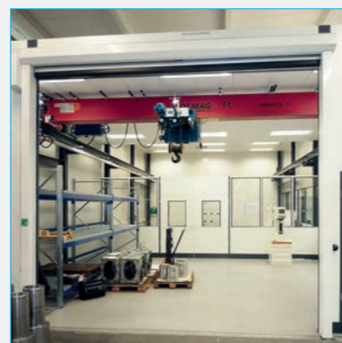
Fully-fledged hall crane use during pre-tempering provided by freezer effect
