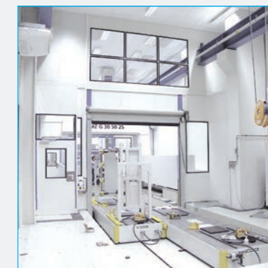
Moving of parts on air cushion system
