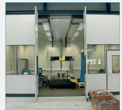
Measuring room with sliding roof
